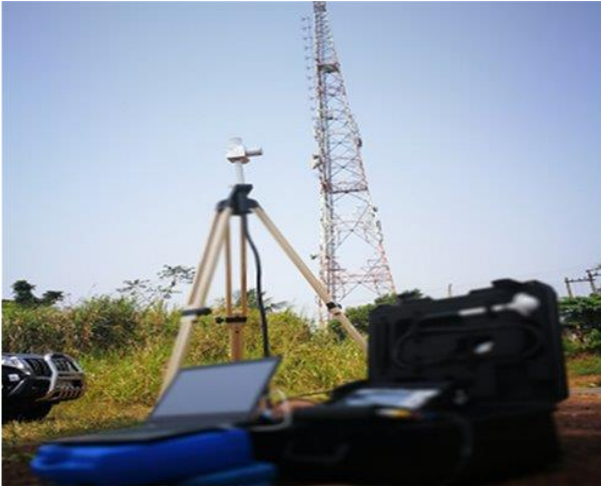
Picture 3: EMF Field Measurement
